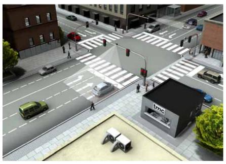
Verification and viewing of the vehicle presence detection zones can be done from the TMC.
